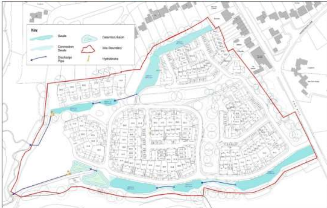
Figure 5-2 - Location of Swales and Detention Basins
